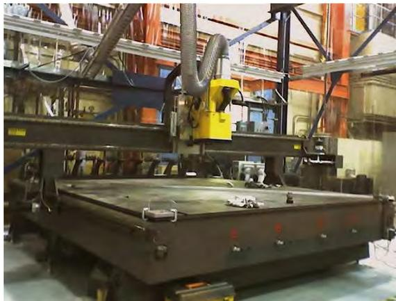
Figure 5.2: Router to be used for much of the TPC mechanical construction at TRIUMF.
