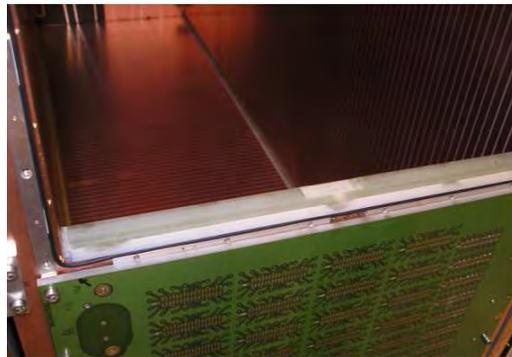
Figure 5.49: (a) A triple GEM structure being attached to the pad board. (b) a view inside the TPC through the hole intended for a GEM amplification module.
