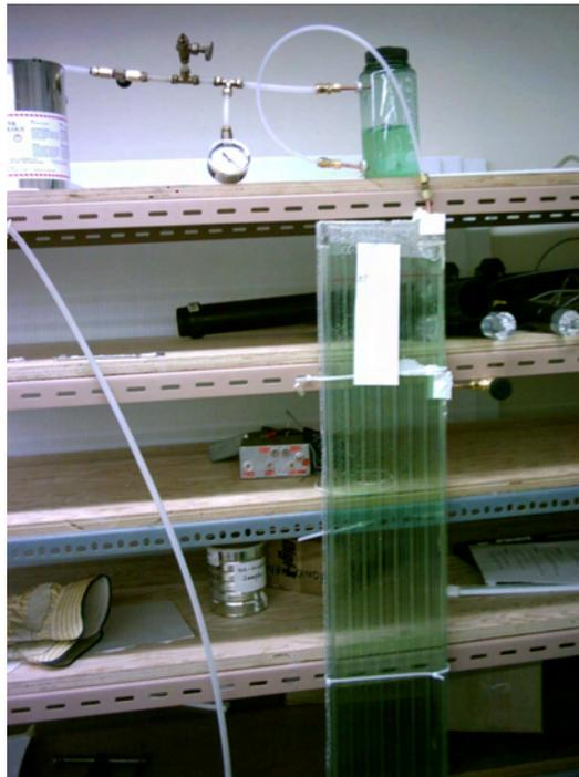
Figure 4.6: Test panel for the target water model. The panel is filled with water (dyed green) under negative pressure. A buffer tank is visible above the panel.
