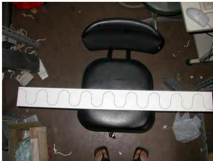
Figure 2.6: A picture of a scintillator strip from the Uniplast Factory at Vladimir in Russia.
