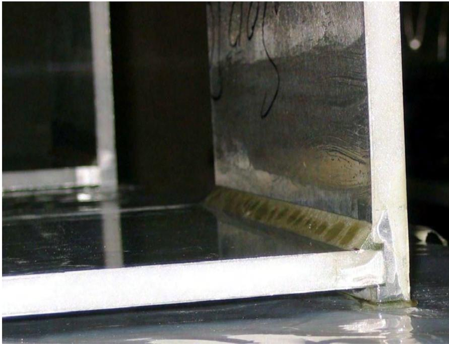
Figure 5.9: Test piece to study the outer box joints, constructed out of aluminum-clad rohocell laminate. In the actual detector, an aluminum frame will cover all rohocell edges.
