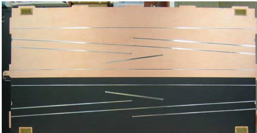
Figure 5.7: The bottom half of the prototype central cathode shows the carbon-loaded kapton with aluminum strips that will be used in the final design.
