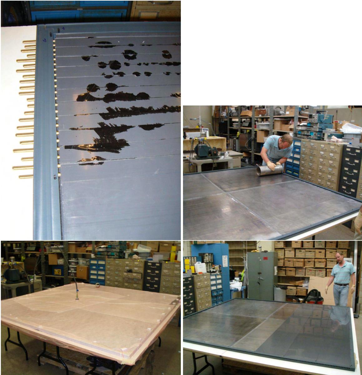
Figure 6.23: (upper left) Brass pins holding a dummy scintillator bar plank into the frame. (upper right) The lead radiator sheet installed into the PØDule during construction. (lower left) A PØDule vacuum-bagged for curing. (lower right) The completed PØDule.
