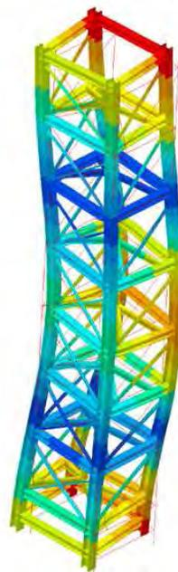
Figure 2.20: Fundamental mode of the tower
