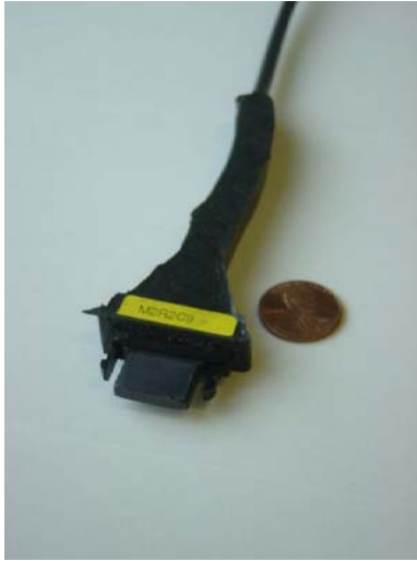
Figure 6.10: The DDK optical connector with light-tight boot made for MINER \nu A.
