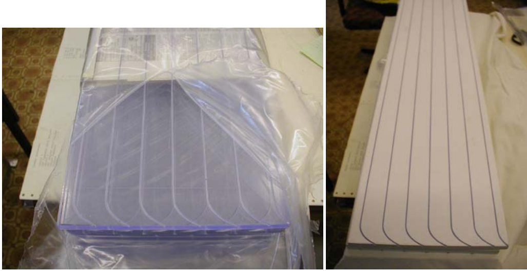
Figure 8.7: The left and right panel show a 87 cm long, 17 cm wide, and 1 cm thick scintillator with grooves to embed WLS fibers. The spacing between the grooves is 2.5 cm. The scintillator shown in the right panel is coated with a chemical reflector.
